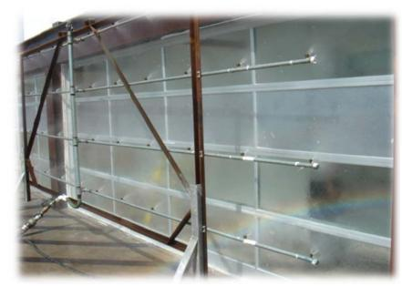
Note: The Water Resistant / Infiltration Package <u>must be</u> <u>combined</u> with the Air Resistant Package <u>DURING THE</u> <u>MANUFACTURING PROCESS</u> to function as tested! This option, <u>CAN NOT BE INSTALLED AFTERWARDS</u>, per the ASTM E331 & ASTM E547 testing standard.
