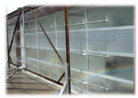
Note: The Water Resistant Package <u>must be combined</u> with the Air Resistant Package <u>DURING THE MANUFACTURING</u> <u>PROCESS</u> to function as tested! The Water Resistant Package <u>CAN NOT BE INSTALLED AFTERWARDS</u>, per the ASTM E331 or ASTM E547 testing standard.
